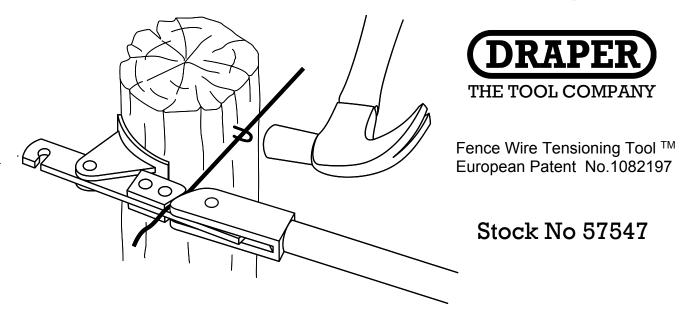
The Fence Wire Tensioning Tool has been designed for simplicity of use and ease of operation. Working from post to post along the fence, it will stretch plain, barbed and stock wire up to  $\varnothing$  4mm and is particularly suitable for quick repairs or when an operator is working alone or in a restricted, sloping or uneven environment.
